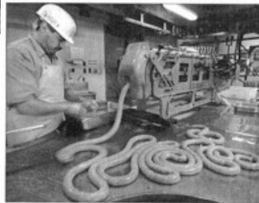
Smear Link when Smear is made of pork sausage into a machine that extrudes into links of Anson's & Sons in San Leandro. At right, Steve Anson's joins sausage into a coil of ground pork that will be turned into links.
