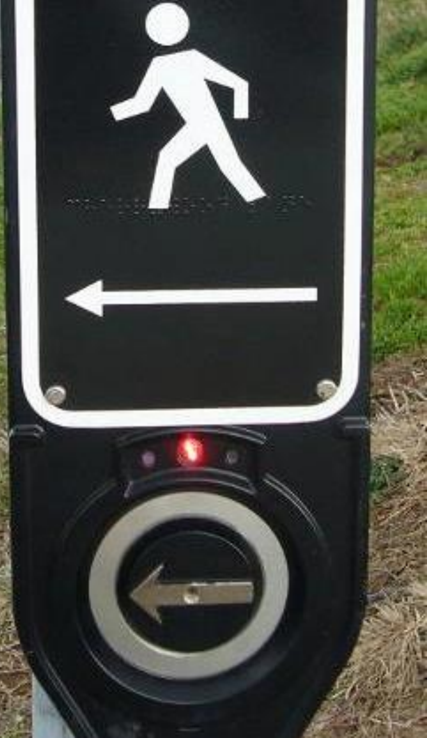
Figure 6-1. Optimal location of pushbutton-integrated APS (two pushbuttons on one corner, mounted on two separated poles " rapid tick WALK indication)
